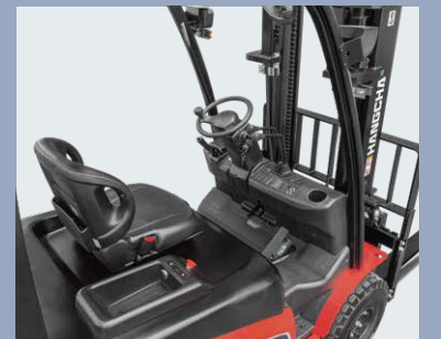
Fully closed operation plate space, tilting cylinder and flat bottom plate, providing more comfortable and safe operation
