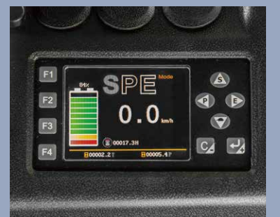
Multi-function instrument with color screen, clear human-computer interaction interface for visualized reading
